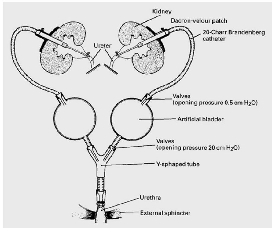
**Fig. 3** The last alloplastic neo-bladder published: the Aachen (Rohrmann) model. Schematic view of two artificial bladders as they were implanted in sheep (from reference [37])
